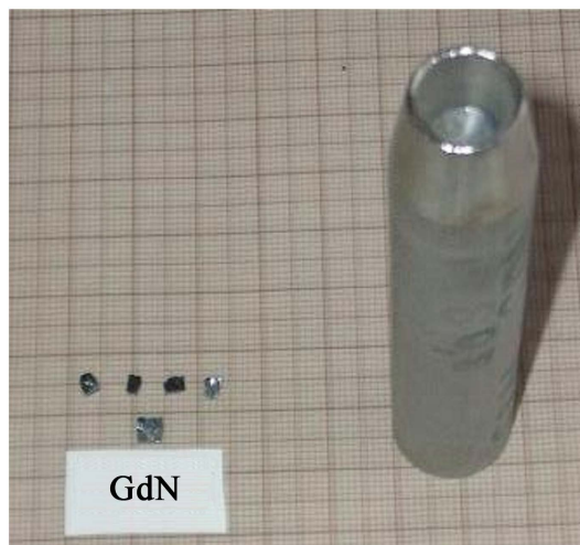
Figure 1. Tungsten crucible (about 10 cm in height) and GdN single crystals.
