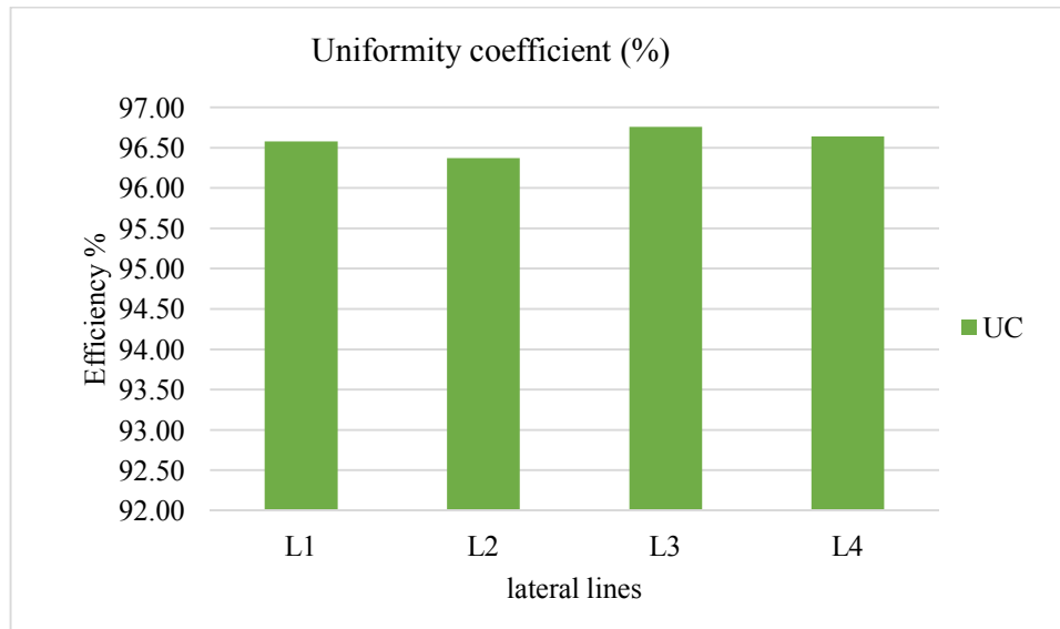
Fig. 4. Uniformity coefficient of different laterals of drip system at operating pressure of 1 kg/cm 2
