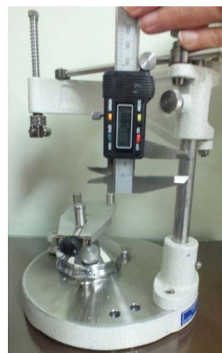
Figure 4. The distance between the two points on the vertical spindle of the surveyor was measured by a digital Vernier device.
