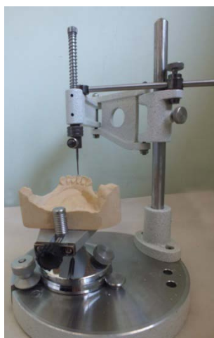
Figure 3. The contact point of the vertical spindle and the cross arm of the surveyor was marked when the analyzer’s tip touched the lowermost point.
