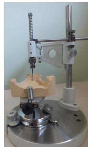
Figure 2. The contact point of the vertical spindle and the cross arm of the surveyor was marked when the analyzer’s spindle touched the lowermost point.
