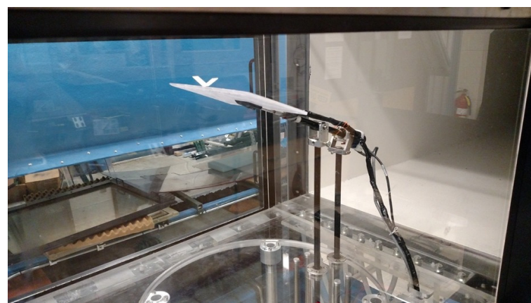
Figure 8. Schematic of the leading-edge alula device adopted by Linehan et al. [22].
