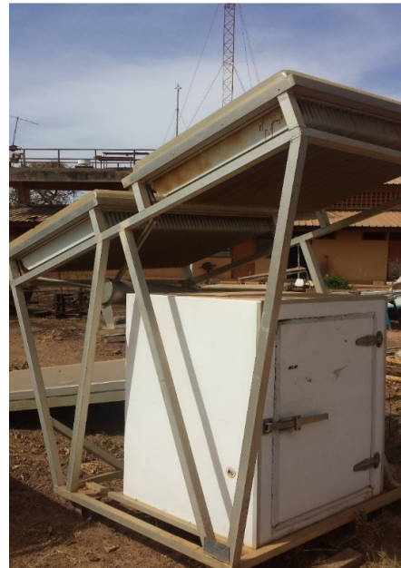
Fig. 2. Photo of the solar refrigerator with silica gel-water couple installed in Ouagadougou
