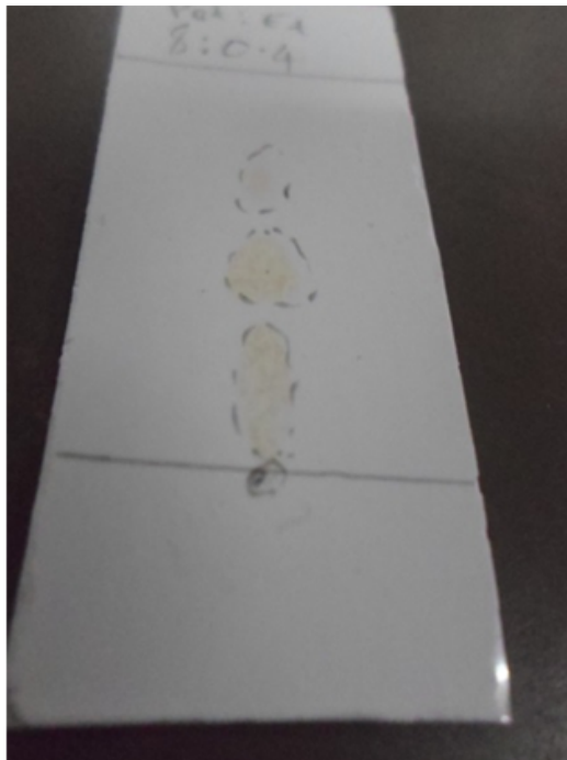
Fig. 2. Crude petroleum ether TLC profile using selected solvent system
