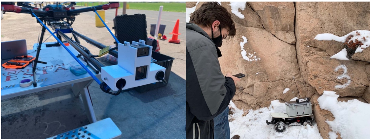
Figure 22. Robotics-based monitoring examples: (left) new aerial system of intelligent measurement integration (NASIMI) [248, 249]; (right) rock-slide detection using machine learning with BRUTUS [250, 251].
