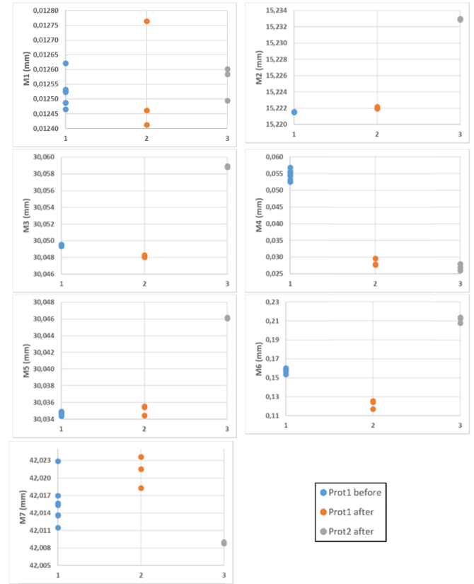
Figure 5. CMM calibration measurements of the CAD Cube implementing protocol 1 (before and after circulation of the CAD Cube) and protocol 2 (after circulation of the CAD Cube) for each measurand.
