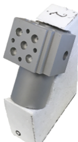
Figure 6. CAD Cube on the holder provided to perform the XCT scans.
