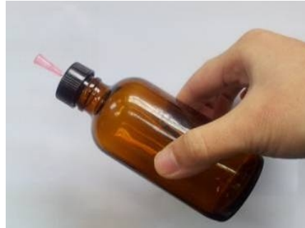
Fig. 5. The dark glass bottle used in the thin-film method
