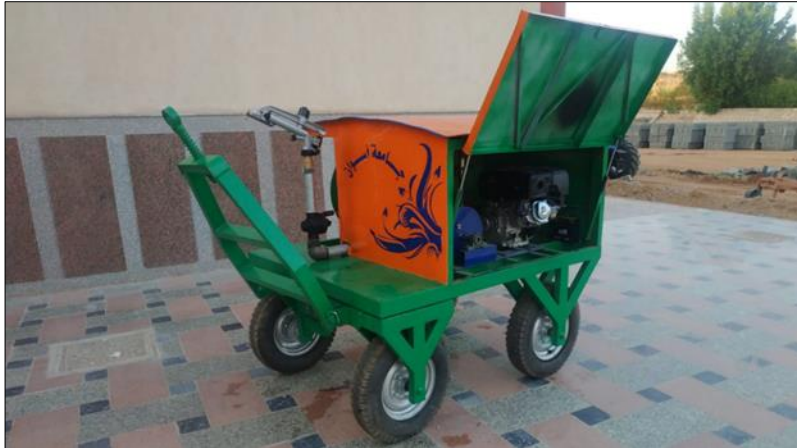
Figure (2): A photo of the prototype self-drawn sprinkler irrigation with opening door.
