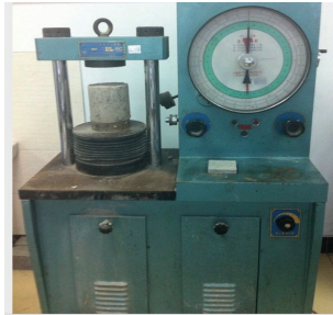
FIGURE 2: Unconfined compressive strength test.
