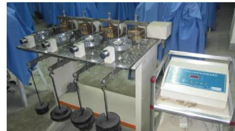
FIGURE 4: STSJ-5 smart electric quadruple direct shear apparatus.
