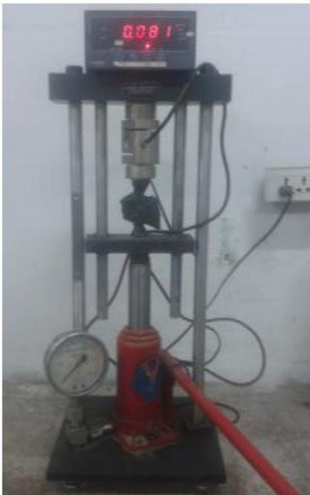
FIGURE 2: Point-load device.
