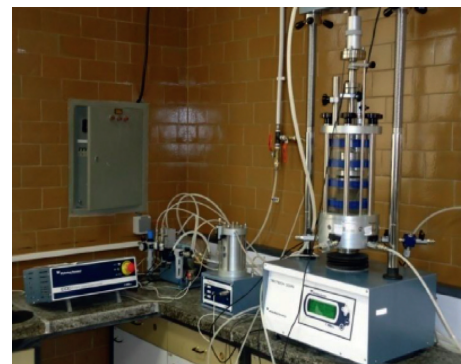
FIGURE 10: GDS high dynamic triaxial testing system.
