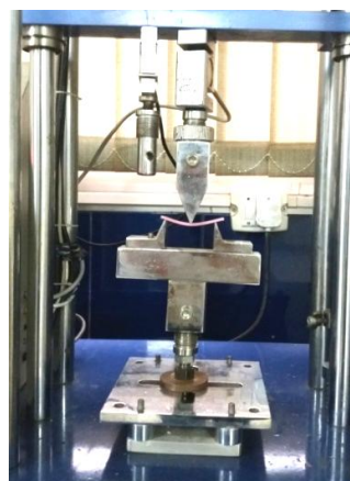
Fig. 2. Testing the specimen on Universal testing machine
