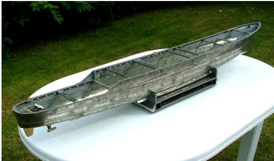
Fig. 23. RC boat hull made from metal [100]
