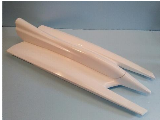
Fig. 24. RC boat hull made from fiberglass [106]
