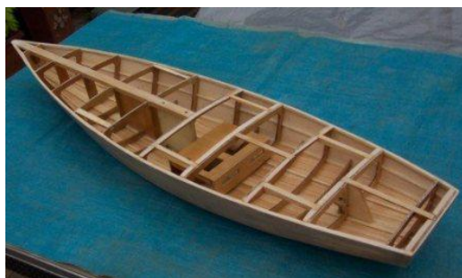
Fig. 22. RC boat hull made from wood [91]
