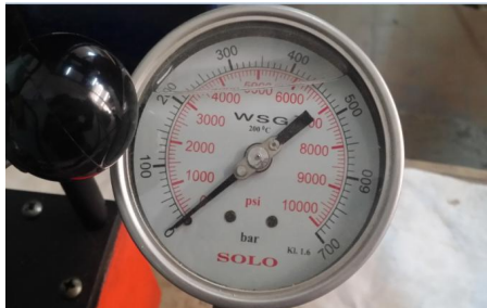
Fig. 7. Dial gauge of the hydraulic jack of loading
