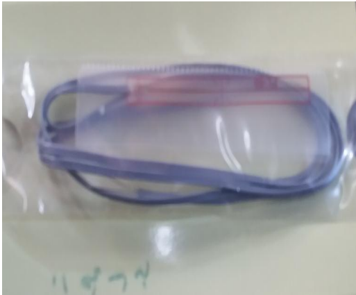
Fig. 3. Applied strain gauges
