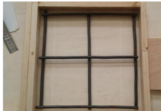
Fig. 5. Square footing model with steel reinforcement
