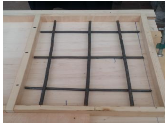
Fig. 4. Rectangular footing model with steel reinforcement
