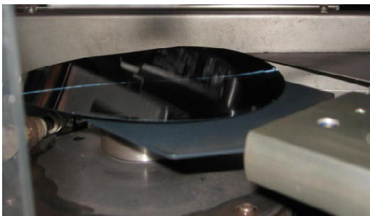
Fig. 7. Vacuum error on the robot arm
