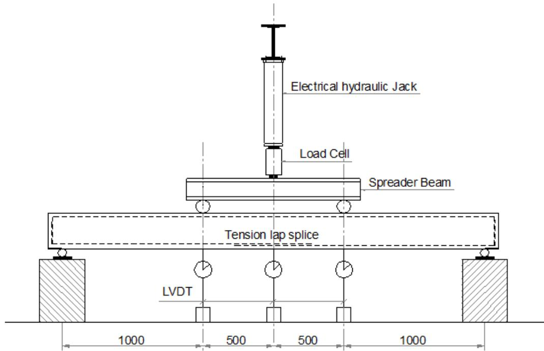
**Fig. 2. Schematic view of the test set-up**
