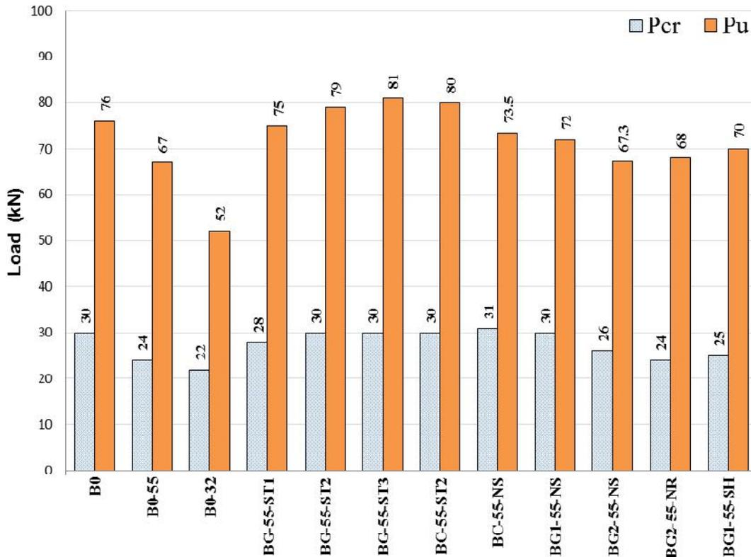
Fig. 14. Cracking and ultimate loads for all beams
