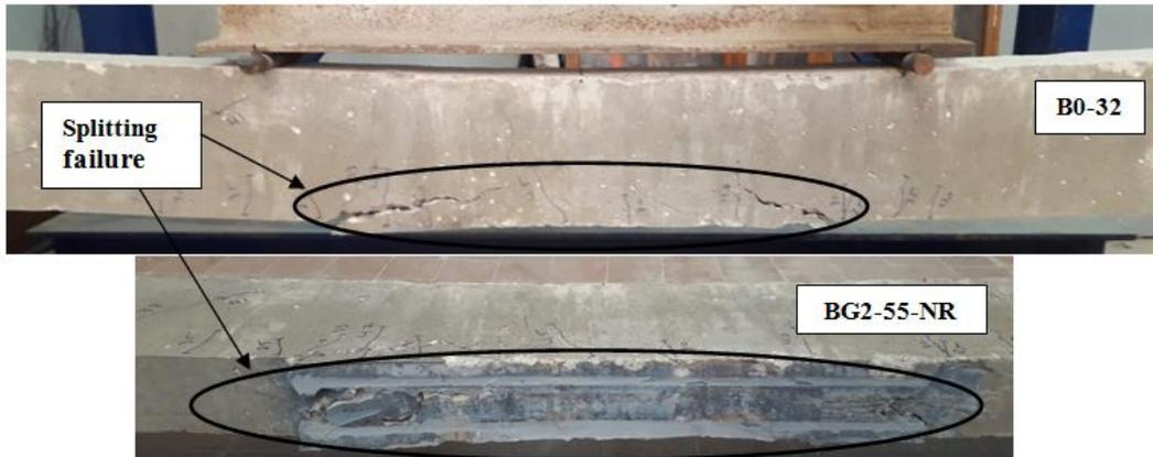
Fig. 6b. Typical splitting (sudden) failure
