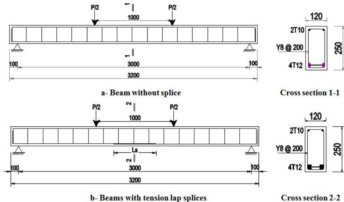
**Fig. 1. Longitudinal and cross section details of beam specimens**
