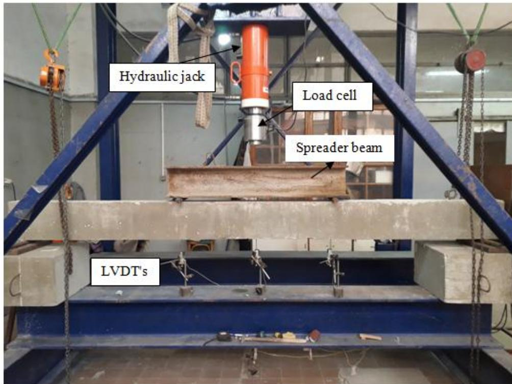
**Fig. 3. Specimen beam prior to the test**
