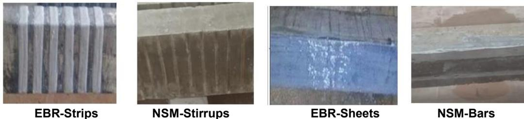
**Fig. 5. Strengthening preparation**
