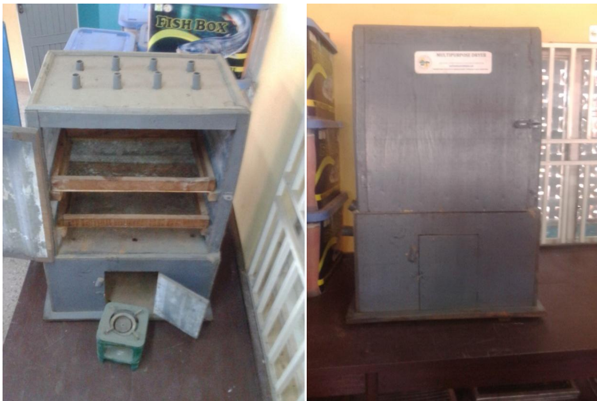
Plate 2/ Open and closed kerosene powered dryer
