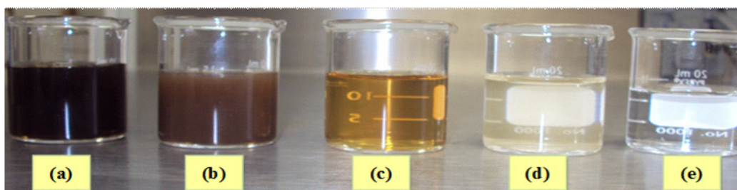
Fig. 14. 14a. Raw leachate (RL), 14b. Leachate pH 3 (AL), 14c. Leachate Fenton oxidized (OL), 14d. Adsorbed leachate OL on eggshell (ESL), 14e. Adsorbed ESL on Active Carbon (ACL), final liquid product
