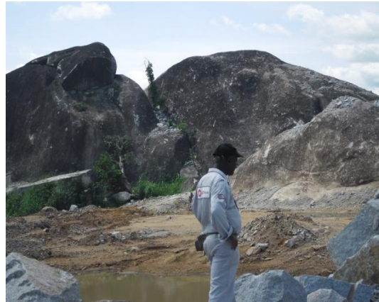
Fig. 8a. Field photograph showing biotite granite with open joints, very important for drilling and blasting for aggregates and dimension stone at Iyuku.
