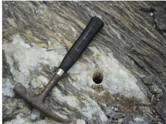
Fig. 6b. Field photograph showing a 5 m hole drilled before blasting at Igue
