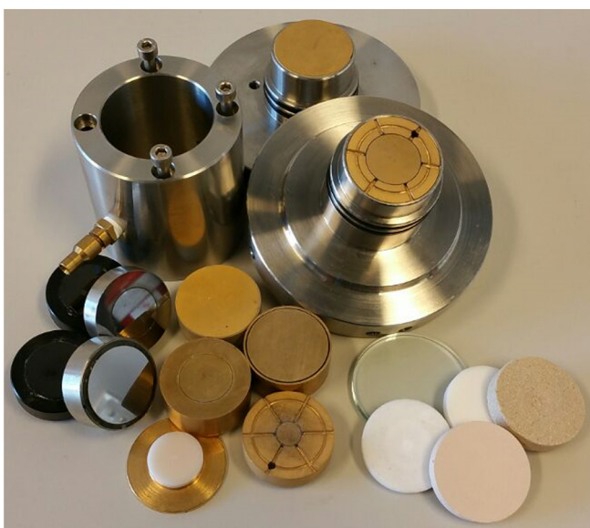
Figure 5. (a) Sketch and (b) photo of the dielectric and acoustic measurement cell. Consisting of a pair of flanges with the detachable measurement platens (orange in the sketch and gold plated brass in photo), which can be re-configured and interchanged for different sample sizes and measurement purposes. Glassy carbon, pyrol and platinum black platens can also be used to overcome electrode polarisation (Ishai et al 2013). The platens may consist of simple dielectric cell modules or combination dielectric-acoustic platens as presented here. The example test samples in the bottom right of the photo include a glass, an alumina and two Teflon standard reference pieces as well as one geological example (Donnybrook sandstone).
