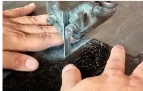
FIGURE 6: Dimensioning and cutting of specimens from the laminates with a DoAll machine.
