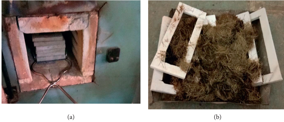
FIGURE 4: Basalt fibers subjected to temperature heating: (a) muffle furnace; (b) fibers removed from muffle furnace after heating.
