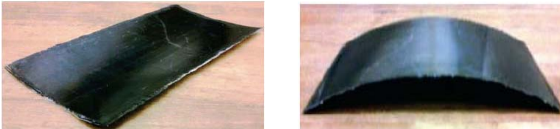
Figure 7. Cured room temperature shapes of [0/90] and [0 2 /90 2 ].
