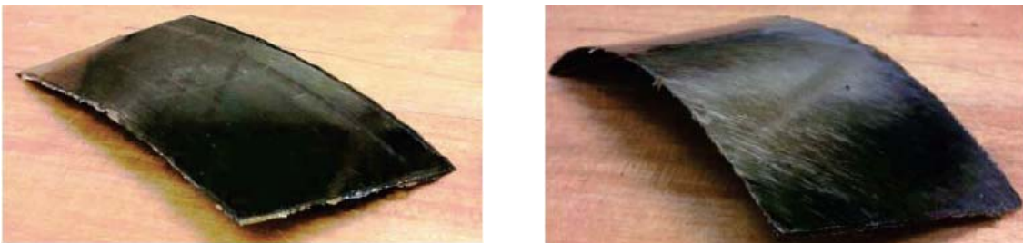
Figure 8. Cured room temperature shapes of [0/45] and [45/90].
