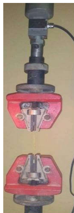
Fig. 1. PALF undergoing tensile testing
