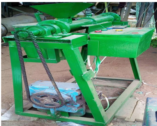
Plate 1. Pictorial view of the modified single screw extruder
